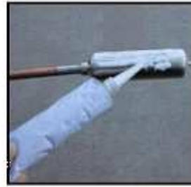
Apply heat conductive paste to condenser for better heat transfer
