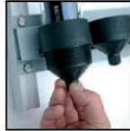
Re-install the retaining cups
